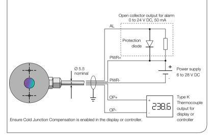
Caution! Check the identification tags and ensure wiring is correct before applying power to the sensor.
