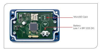
Data is saved to the MicroSD Card in .csv format. This file format can be opened or imported by spreadsheet software such as Microsoft Excel.
