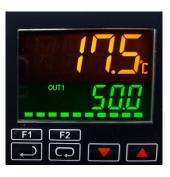
The ThermCal400 controller offers a large, bright and easy to read display. This controller has advanced 5 zone PID control for optimum performance and adjustable ramp rates for proper testing of thermal switches. The unit is switchable between °F and °C along with the ability to easily adjust unit calibration using your own temperature standards.
