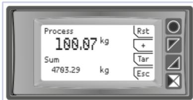
Press "Sum Function" to enter the function page. Pressing "+" the **Process** value is added to the counter. It is possible to reset the total value keeping pressed "Rst" and to fix "tare zero" of the process pressing "Tar".
