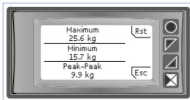
The STR551 is provided with a page for the visualization of peak values: max. peak, min. peak and peak-to-peak of analogue input. Keeping pressed “Rst” it is possible to reset the visualized values.
