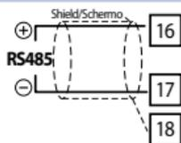
RS485 Modbus RTU communication
