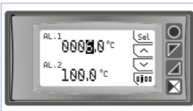
Press "Setpoint" to enter the thresholds modification.
