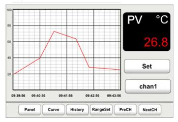
By pressing the Operation button, you will enter the single channel display screen which will provide a graph and meter display of that single channel. You can also enter this screen by pressing on the channel label from the Panel Meter screen. Once in the single channel display screen, press the Set button to display a screen which will allow the high and low alarm values (HIAL, LOAL), the process value offset (Scb) and the alarm hysteresis(HYS) to be set.
