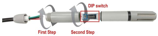
The above figure is a diagram of the correct steps to open the sensor body to expose the DIP switch.
