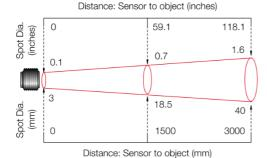
Diagrams show the diameter of the measured spot at each distance, for 90% energy.
