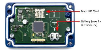
The MicroSD Card and battery slots are located on the touch screen circuit board. Unscrew the lid of the electronics module to access them.
