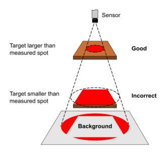
The size of the area (spot size) to be measured determines the distance between the sensor and the target. The spot size must not be larger than the target. Choose a suitable mounting distance so that the measured spot size is smaller than the target.
