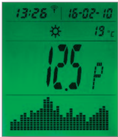
Up to the minute cost information – this screen shows real time spending of 12.5p per hour
