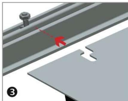
**INSTALL MICROINVERTER:** Install microinverter on to rail. Engage with bolt.
