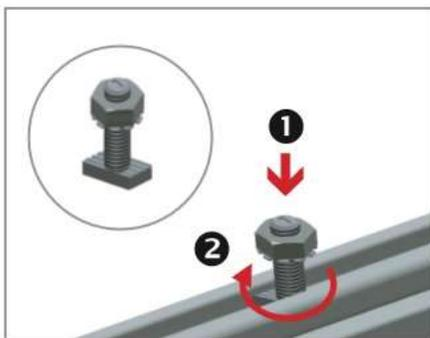
**INSTALL MICROINVERTER MOUNT T-BOLT:** Apply Anti-Seize and install pre-assembled 1/4" dia. bonding T-bolts into top 1/4" rail slot at microinverter locations. Rotate bolts into position.
