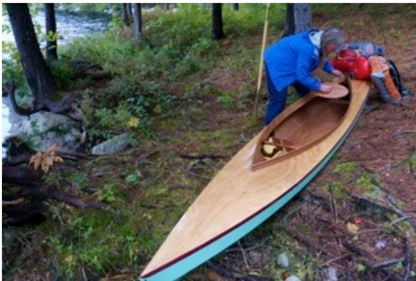
built stitch & glue with 6oz fiberglass cloth on the bottom and a cambered deck. The 2 bulkheads have hatches for access to the dry storage areas behind them and create positive flotation chambers.
