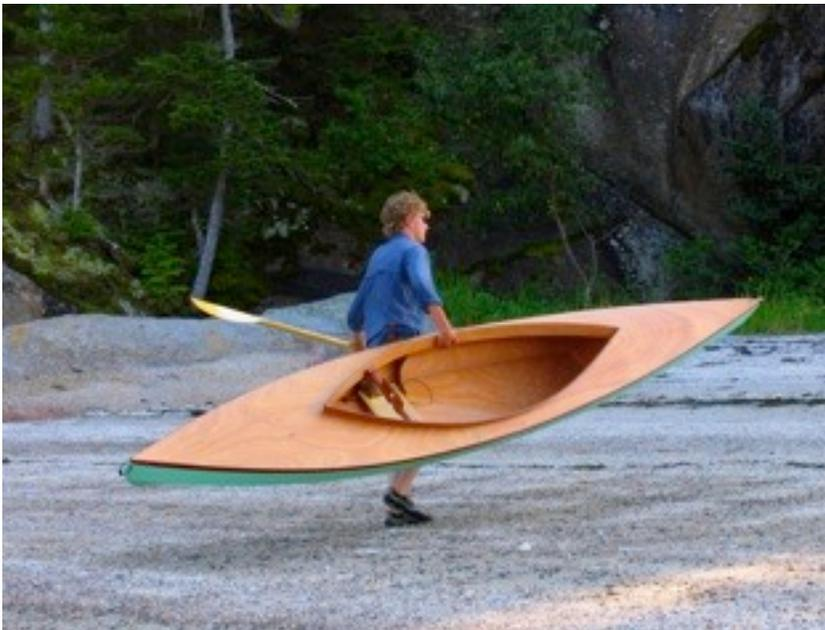
My Fox design, at 14'7" is longer than most decked canoes and the beam of over 30" adds greatly to the stability and capacity of the boat. At about 44 pounds it can easily be carried on one's shoulder and is stable enough to step into at the waters edge. It is possible to simply walk down to an inviting lake or marsh and slip Fox into the water for an afternoon of casual paddling and exploration.
