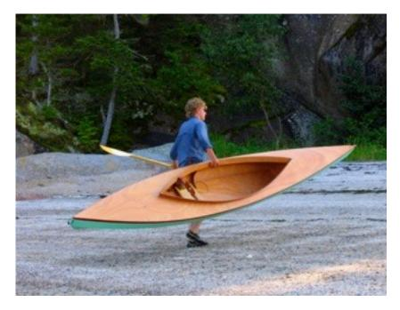
My Fox design, at 14'7" is longer then most decked canoes and the beam of over 30" adds greatly to the stability and capacity of the boat. At about 44 pounds it can easily be carried on one's shoulder and is stable enough to step into at the waters edge. It is possible to simply walk down to an inviting lake or marsh and slip Fox into the water for an afternoon of casual paddling and exploration.
