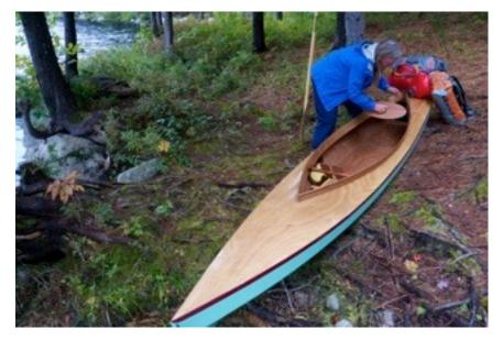
chop or swell. Fox is built stitch & glue with 6oz fiberglass cloth on the bottom and a cambered deck. The 2 bulkheads have hatches for access to the dry storage areas behind them and create positive flotation chambers.
