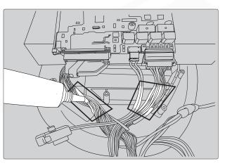
18. Insert the Immobilizer Control Unit into the Waterproof Case. The black connector on the Immobilizer has to fit into the 2 alignment pins built into the Waterproof Case.
