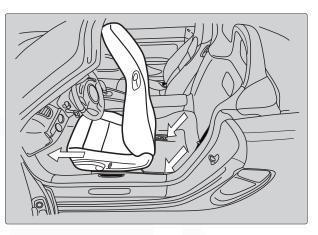
2. Move the seat all the way back, and take off the 2 plastic covers on the seat rails that are held by phillips head screws.
