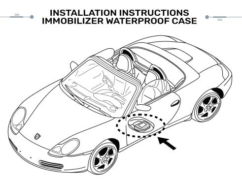
All Porsche Boxsters and 911 models that were made from 1997 through 2005 have a weakness in the location of the Immobilizer Security System. This computer was placed directly onto the floor of the car, under the driver's seat, making it prone to getting water damaged.
