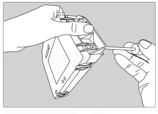
7. Insert the right side bottom lip of the waterproof case in the hole of the floor of the chassis.
