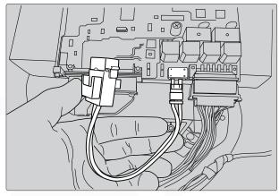
13. Insert the 15 amp fuse inside the fuse socket of the extension.
