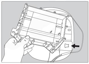
8. Secure to the floor the left side of the case with the plastic locking screw you saved earlier.
