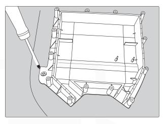
9. Put a liberal amount of silicone sealant in the 2 dams of the bottom of the case. This will help the sealant to spread between the cables of the harness when you close the case with the top lid.
