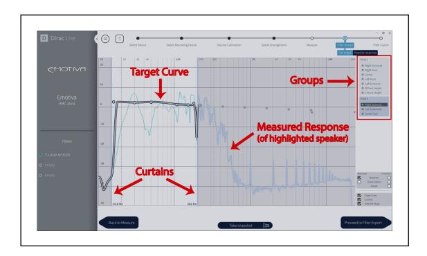
Dirac Live room correction works by using a series of test tones to measure the frequency response of your system and room, analyzing the results, comparing them to a desired frequency response Target Curve, and calculating a set of Correction Filters that will adjust the frequency response of your system and room so that it matches the Target Curve. (Dirac Live also performs calculations that enable it to correct phase anomalies as well as variations in frequency response.)
