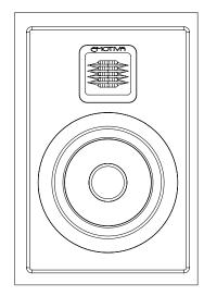
The Airmotiv XB2 is a two way monitor loudspeaker, equally at home on a sturdy bookcase or stand, featuring a 28x32 mm Airmotiv folded ribbon tweeter and a 6 inch woven fiber woofer. The Airmotiv XB2 is ideal for use in a small, high-quality two-channel system, and has plenty of low frequency output to sound great in a small room without the need for a subwoofer. The Airmotiv XB2 also works well as a surround speaker in a home theater system where you prefer not to use wall-mounted speakers.
