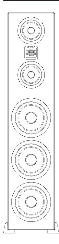
The Airmotiv XT3 is a three way, floor standing, tower loudspeaker, featuring a 28x32 mm Airmotiv folded ribbon tweeter, dual 5-1/4 inch woven fiber midranges, and three 8 inch woven fiber woofers. The Airmotiv XT3 can be used in an audiophile stereo setup, or as a main front speaker in a home theater installation, or you could use a full set of Airmotiv XT3's as the basis of an unsurpassed home theater installation.
