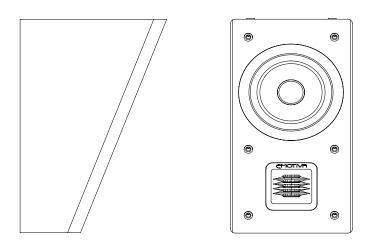
The Airmotiv XA2 is a two way loudspeaker, featuring a 28x32 mm Airmotiv folded ribbon tweeter and a 5-1/4 inch woven fiber woofer, which can be used as a wall mounted direct firing surround sound or height channel speaker, or as a ceiling mounted direct firing height speaker.
