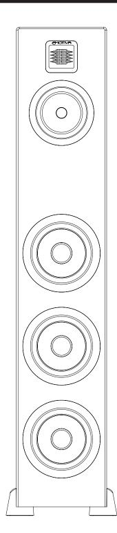
The Airmotiv XT2 is a three way, floor standing, tower loudspeaker, featuring a 28x32 mm Airmotiv folded ribbon tweeter, a 5-1/4 inch woven fiber midrange, and three 6 inch woven fiber woofers. The Airmotiv XT2 can be used in an audiophile stereo setup, or as a main front speaker in a home theater installation, or you could use a full set of Airmotiv XT2's as the basis of a really high end home theater installation.
