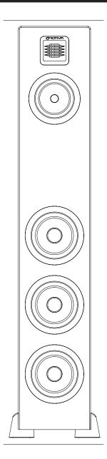
The Airmotiv XT1 is a three way, floor standing, tower loudspeaker, featuring a 28x32 mm Airmotiv folded ribbon tweeter, a 4-1/2 inch woven fiber midrange, and three 5-1/4 inch woven fiber woofers. The Airmotiv XT1 can be used in an audiophile stereo setup, or as a main front speaker in a home theater installation, or you could use Airmotiv XT1's all around in a high end home theater installation.
