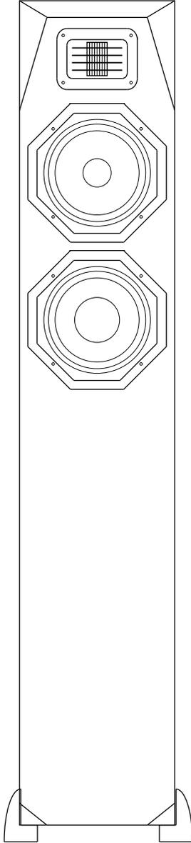
The Airmotiv T0 is a two way, floor standing, tower loudspeaker, featuring a 32mm Airmotiv folded ribbon tweeter, and a pair of 5-1/4" woven fiber drivers. The dual 5-1/4" drivers share the same 2500 Hz electrical crossover frequency, but the upper one is optimized for the critical midrange frequencies, while the lower one is optimized for low frequency response. The Airmotiv T0 is ideal for any stereo or home theater system where both excellent sound quality and a compact footprint are needed.
