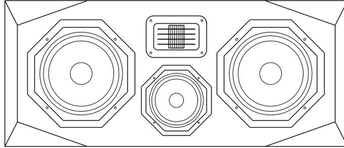
The Airmotiv C1 is a three way center channel loudspeaker, featuring a 32mm Airmotiv folded ribbon tweeter, a 3" woven fiber midrange, and dual 5-1/4" woven fiber woofers. The Airmotiv C1 is designed to be used as a center channel speaker in high end home theater installations.
