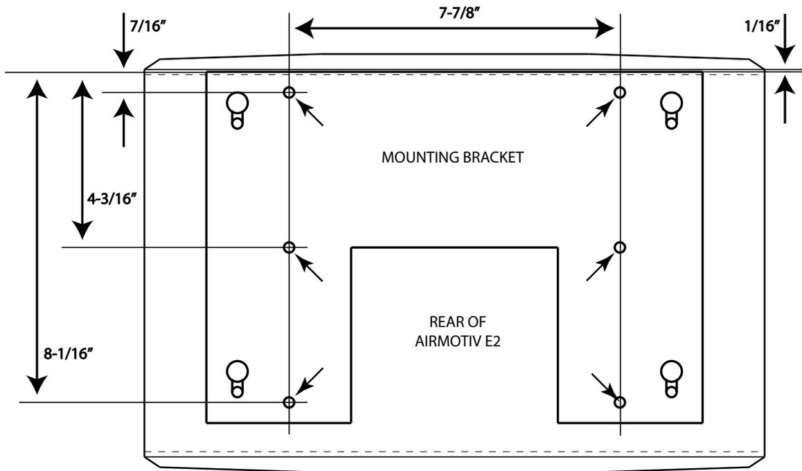
Note six (6) wall bracket mounting holes.
