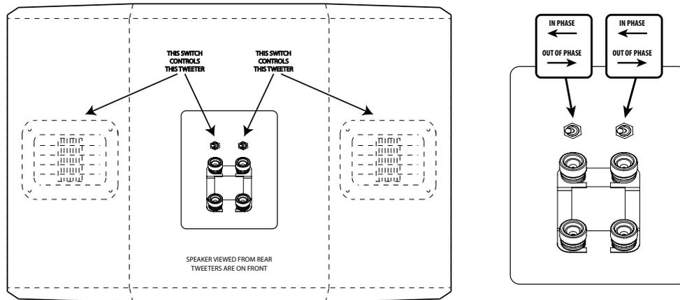
The Airmotiv E2 will provide the most precise sound imaging and localization when configured as a conventional direct firing or “bipole” surround speaker, and this is what most modern surround sound standards recommend. To configure the Airmotiv E2 for this mode, simply set both switches on each Airmotiv E2 to IN-PHASE.
