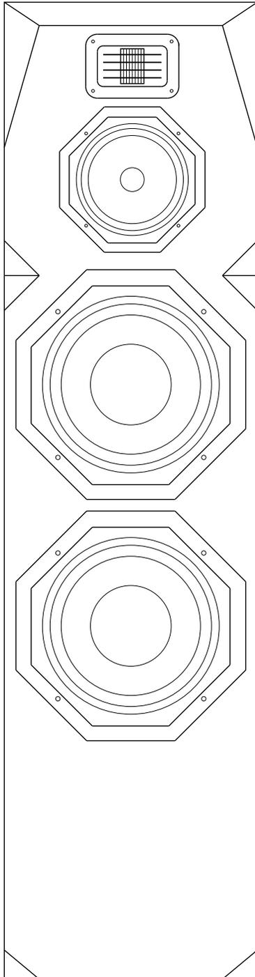
The Airmotiv T2 is a three way, floor standing, tower loudspeaker, featuring a 32mm Airmotiv folded ribbon tweeter, a 5-1/4" woven fiber midrange, and dual 8" woven fiber woofers. The Airmotiv T2 can be used in an audiophile stereo setup, or as a main front speaker in a home theater installation, or you could use a full set of Airmotiv T2's as the basis of a really high end home theater installation.
