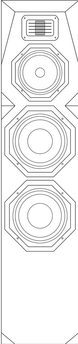
The Airmotiv T1 is a three way, floor standing, tower loudspeaker, featuring a 32mm Airmotiv folded ribbon tweeter, a 5-1/4" woven fiber midrange, and dual 6" woven fiber woofers. The Airmotiv T1 can be used in an audiophile stereo setup, or as a main front speaker in a home theater installation, or you could use Airmotiv T1's "all around" in a high end home theater installation.
