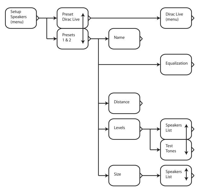
The Setup Speakers Menu is where you access the powerful speaker and room correction features of the XMC-1, including Dirac Live automatic room correction, and the XMC-1's incredibly flexible manual calibration system, which includes two fully independent banks of parametric equalizers, along with pink noise and test tone generators.
