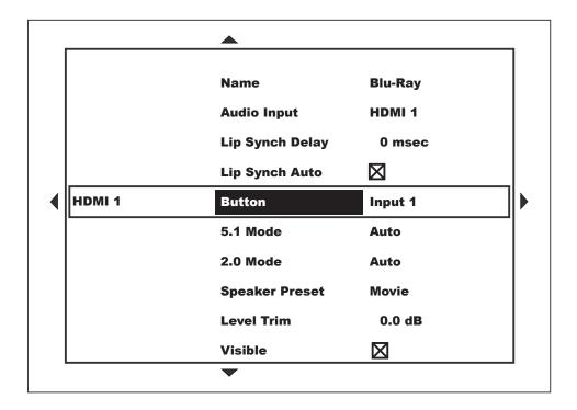
The Menu System is entered by pressing the Menu button on the XMC-1's front panel, or on the remote control; pressing the button a second time, or pressing the Left arrow button when you are already at the top level of the menu, exits the menu and returns you to the Information Screen. Menu navigation is accomplished using the Up, Down, Left, Right, and Enter buttons on the front panel or the remote control.
