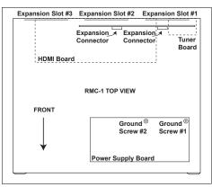
Note: If you are installing a single module you will find that Slot #1 is easier to access without removing other components. You may find that Slot #2 is easier to access if you remove the HDMI board first (optional).
