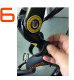
Wrap the clamp around the handlebar stem.
