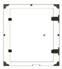
Attach the doorknob by first inserting the square M4 nut into the slot. Use a 16mm cap head screw to attach the door.
