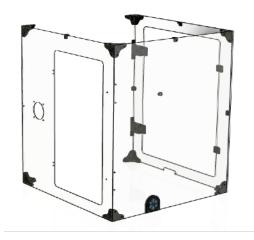
Next, assemble the back door using the same techniques as the front door, i.e., hinges, latch mounts, and strike plates. The main difference is that the strike plates will need to be squeezed in to fit the smaller thickness of the back panel v.s. The front panel.
