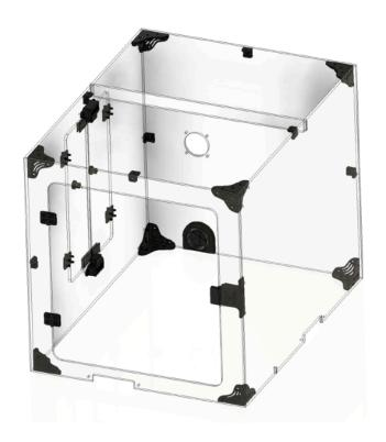
Use access through the doors to attach the top of the enclosure using M4 12mm screws. You'll attach the top on the four corners, and to each of the mid-panel connectors as well. The slit is towards the front, and the small access hole for the filament runout sensor cable should be on the right. The view shown at the right is from above facing the front of the printer.
