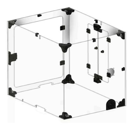
Attach the right panel as shown above at each of the four corners. You can now attach the latch mount on the front using 2 M4 12mm cap head screws.
