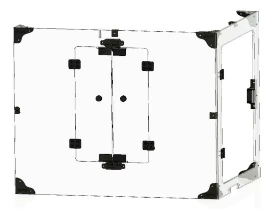
Attach the left side to the front forming an L-shape that will stand up on its own, then attach one L and one R connector at the back. The Ender 3 S1 design technically doesn't need a door, but it allows for additional access to the extruder. The latch mounts are smaller than the front, although the magnetic latch attaches in the same way with wood screws. The parts for the side door will be in a separate packet.
