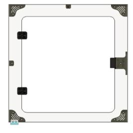
Now that the latches are mounted it is time to connect the strike plates. Each plate comes with a squishy adhesive covering the same size of the plate. Carefully attach the adhesive side to the
