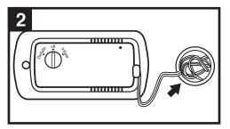
Once air mattress is completely deflated, turn control dial clockwise to the "Off" position and place cord in the "Cord Storage Pocket".
