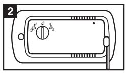
Upon reaching desired firmness turn the control dial counter-clockwise to the "Off" position. Make sure the switch aligns with the "Off" arrow. Air mattress is now ready for use.
