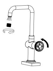
Remove aerator assembly (1) from faucet body (2). Turn faucet on and let the water run for 60 seconds to flush any debris.
