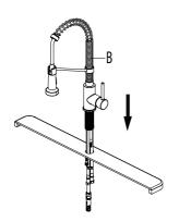
Shut off the water supply. Insert faucet body (B) through the hole inthe sink.
