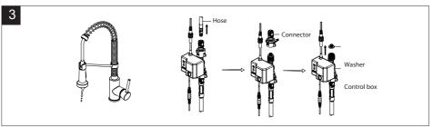
a. This could indicate that the washer in the control box is dirty or damaged. Remove the hose and unscrew the connector. Take out the washer from the control box. Clear the washer or replace the washer. Reassemble the
