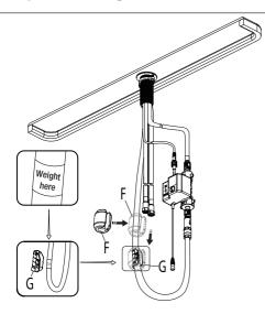
Install the weight clip (G) at the point of the hose marking "weight here". Insert the weight (F) onto the weight clip (G) by sliding it down onto the weight clip (G).
