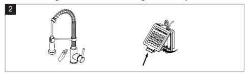
If the handle is closed, turn the handle to the on position and move your hand in the sensor area. If the sensor flashes 10 times continuously and slowly, then replace the 4 "AA" batteries.
