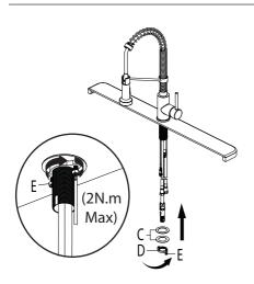
Install the washers (C) onto the threaded mounting shank.
