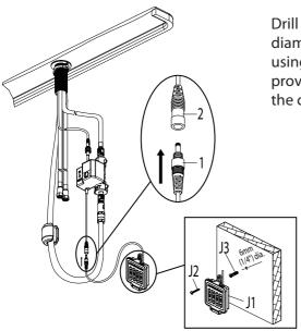
Drill a hole in the wall using a 6mm (1/4 in.) diamater drill bit. Install the battery pack (J1) using the molly anchor (J3) and screw (J2) provided. Insert the battery pack cable (1) into the control box connection (2).
