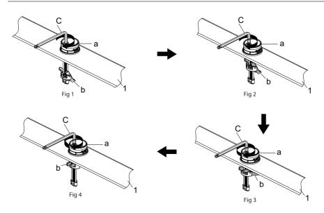
Press the base (a) so that it can not move, then turn the screw with the provided hex wrench (C, HEX: 6.0mm) clockwise, as shown Fig 1. When the mounting plates (b) make contact with the sink (1), continue to turn the screw with the provided hex wrench (C, HEX: 6.0mm) clockwise, as shown Fig 2, until the base (a) is completely tightened and secured, as shown Fig.4.
