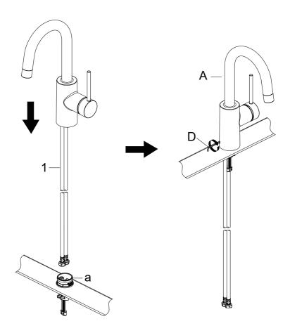
Insert the supply lines (1) through the hole of the base (a). Carefully insert the hoses into the base. Place the faucet assembly (A) onto the base (a) as shown in the above figure. Secure the faucet assembly (A) by tightening the set screw with the provided hex wrench (D, Hex: 2.5 mm).
