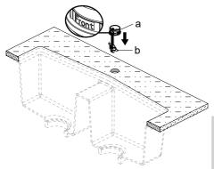
Shut off the water supply. Remove the old faucet. Clean the mounting surface. Check for the proper thickness of the sink. Insert the base (a) into sink.
