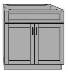
The cabinet on the left is made for an apron sink. This is called a country sinkbase cabinet. Note the shorter doors. The space taken from the height of the doors is given to the space occupied by the height of the apron sink face,
