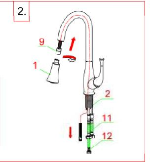
Connect spray(1) and spray hose(9). Insert spray hose through the main body. Connect and tighten inlet hoses (11) and connecting hose(12) onto the main body.
