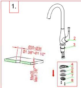
1.Before installation, be sure of the indicated thickness and hole of intallation board. Remove the bolts(8), nut(7), matel gasket(6), washer 2(5) and plastic gasket(4) from the main body(2).
