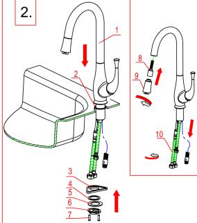
Connect spray(9) and spray hose(8). Insert spray hose through the faucet. Connect and tighten water supply hoses (10) to the faucet main body. Insert the faucet with washer 1 (2) through the faucet hole. Install plastic gasket(3), washer2 (4), clamping ring(5), nut(6) and screws(7).
