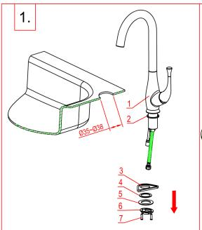
Check the thickness of the installation surface and make a faucet hole according to above fig.
