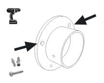
Move unit away from wall and remove wall flange from tube and mount flange to wall using  $12 \#10 \times 1\frac{1}{2}$  in. wall mount flange screws **(#3)** and plastic wall anchors **(#4)** if needed.
