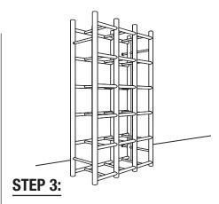
Turn unit upright and place firmly against wall where unit is to be mounted.
