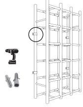
Note: If mounting into drywall or masonry, mark and drill ¼ holes and insert plastic wall anchors – and proceed with the previous step.
