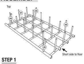
18 Horizontal slide rails (#7) inserted and 4 front and rear grid connecting tubes (#5) inserted in rear grid.
