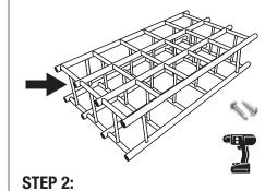
Insert and fasten 18 horizontal slide rails (#7) into front grid assembly using  $18 - \#06 \times \%$  in. fastening screws (#1). Note: Fasteners in bottom hole only, work from bottom row to top row.
