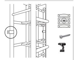
Place 4 wall mount bracket (#06) over 4 rear verticals above  $2^{nd}$  horizontal crossbar (#1) and fasten to wall using  $8 - \#10 \times 1\frac{1}{4}$  in. fastening screws. (#2).
