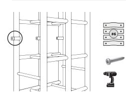
Place 4 wall mount bracket (#06) over 4 rear verticals above 2<sup>nd</sup> horizontal crossbar (#1) and fasten to wall using  $8 - #10 \times 1\frac{1}{4}$ fastening screws. (#2).
