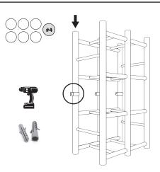
Note: If mounting into drywall or masonry, mark and drill 1/4 holes and insert plastic wall anchors - and proceed with step 1 - Insert decorative top caps (#4) into all verticals.
