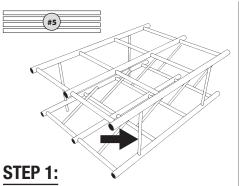
Join front to rear grid by inserting 4 front & rear grid connecting tubes (#5) into front grid assembly Note: Do not fasten at this time
