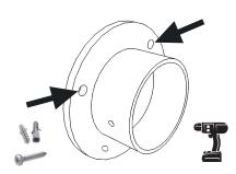
Move unit away from wall and remove wall flange from tube and mount flange to wall using 12 #10 x  $1\frac{1}{2}$  in. wall mount flange screws (#3) and plastic wall anchors (#4) if needed. Note: If mounted into masonry or drywall, drill three  $\frac{1}{4}$  in. holes to accept plastic wall anchors.
