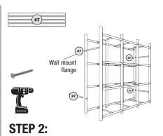
Move unit away from wall and insert 4 wall mount extensions tubes (#7) in 4 locations. Fasten with  $8 - #08 \times \frac{3}{4}$  in. extension tube fastening screws (#2). Note: One fastener per joint front side only.
