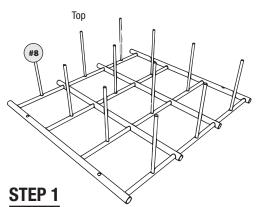
12 Horizontal slide rails (#8) inserted in rear grid.
