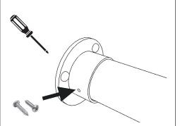
Slide unit back against wall while inserting all 4 wall mount extension tubes (**#7**) into wall mount flanges (**#6**) and fasten with 4 -#06 x  $\frac{1}{2}$  in. fastening screws. (**#1**).
