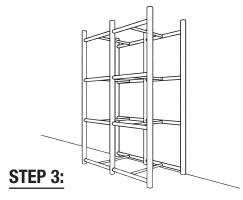
Turn unit upright and place firmly against wall where unit is to be mounted.
