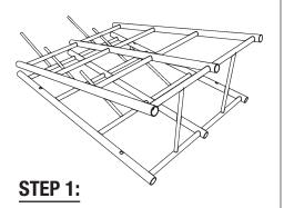
Insert bottom slide rails (#8) into front grid assembly and fasten (making sure fully inserted) using  $2-\#08 \times 3\%$  in. fastening screws (#1) Note: Fasteners in bottom hole only
