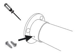
Slide unit back against wall while inserting all 4 wall mount extension tubes **(#7)** into wall mount flanges **(#6)** and fasten with  $4 - \#08 \times 3\%$  in. fastening screws. **(#1)**.
