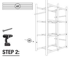
Move unit away from wall and insert 4 wall mount extensions tubes **(#7)** in 4 locations. Fasten with  $8 - \#08 \times 1-\frac{1}{2}$  in. extension tube fastening screws **(#2)**.
