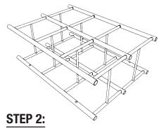
Insert and fasten next 3 rows of slide rails to front grid using  $6-\#08 \times 3/4$  in. fastening screws **(#1)**
