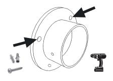
Move unit away from wall and remove wall flange from tube and mount flange to wall using  $12 \#10 \times 1\frac{1}{2}$  in. wall mount flange screws (#3) and plastic wall anchors (#4) if needed. Note: If mounted into masonry or drywall, drill three  $\frac{1}{4}$  in. holes to accept plastic wall anchors.
