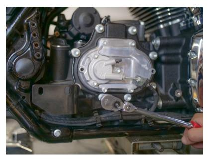
(2). Install mounting bracket using two head cap screws previously removed from stock. Use some type of locking glue, install as shown using a 1/4" hex key wrench.
