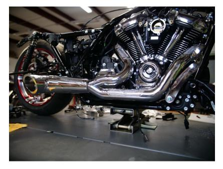
(15). Clean exhaust system with some chrome cleaner and remove painters tape (if used during installation) before turning on engine. Failure to follow this procedure may result in damage to the chrome finish as oils burn out leaving permanent marks.
