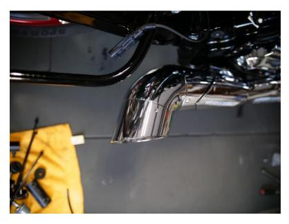
(10). Most systems are shipped with end caps and turn out already installed, if this is not the case proceed to install turn out and end cap.
