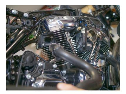
(5). Install headers/muffler assembly into exhaust port by first and carefully aligning the flange holes with the studs on the engine port. Secure it with stock flange nuts using a 1/2" socket and bring nuts all the way finger tight but DO NOT TIGHTEN AT THIS TIME YET.
