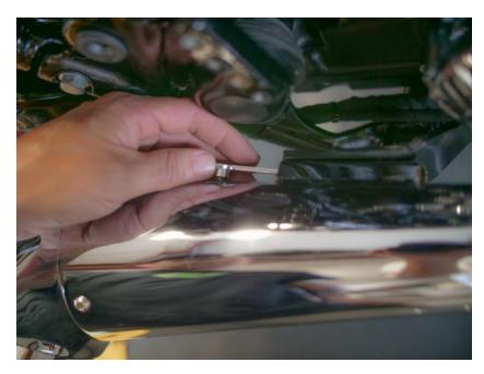
(6). Secure muffler to mounting bracket using a back plate bracket and two 5/16" -  $18 \times 5/8$ " serrated flange screws. Finger tight all the way.
