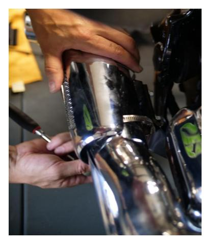
(8). Install heat shields. Start with front shield first. Place front shield over front pipe and insert hose clamps carefully looping the tail of clamp and engaging the welded clip inside shield. Use #24 hose clamp. Use a 5/16" nut driver but do not tighten at this time.
