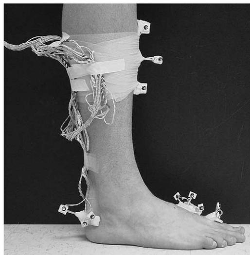
**Fig 3.** Sensors for the Optotrak Motion Analysis System.
