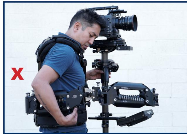
With the X3 held just above horizontal, you'll feel the knob unlock. Adjust the X3 lift to support your rig and 2-section arm.
