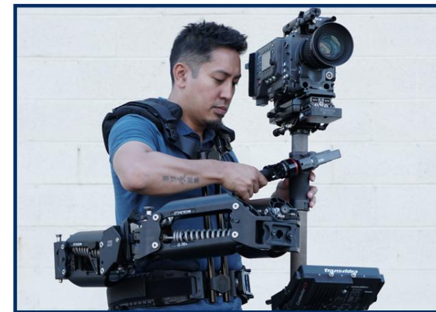
To make a fore-aft adjustment, loosen the top knob, make your adjustment with the lower knob and re-snug the top.
