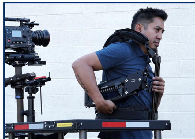
Hold onto the arm section with your right hand as you climb in, lifting the shoulders into place with your left. Secure the shoulder dovetail and then move on to the waist.
