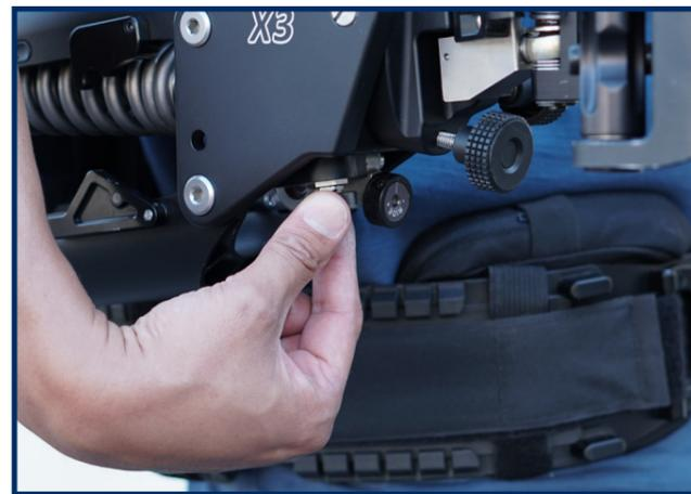
The side-to-side adjustment rotates the socket block similar to the fore-aft adjustment on a traditional mount.
