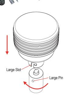
2. Index the bulb so the large slot on the socket of the bulb lines up with the large pin on the lamp plug.
