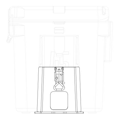
Lift your A45 or A75 APEX Cooler above the Hitch Rack and slide the Wings into the grooved cooler sides.
