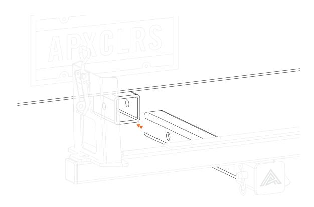
Slide the end of the Receiver Tube into your vehicle's Receiver Hitch. The hitch pin holes on the Receiver Tube should align with the hitch pin holes on the Receiver Hitch.
