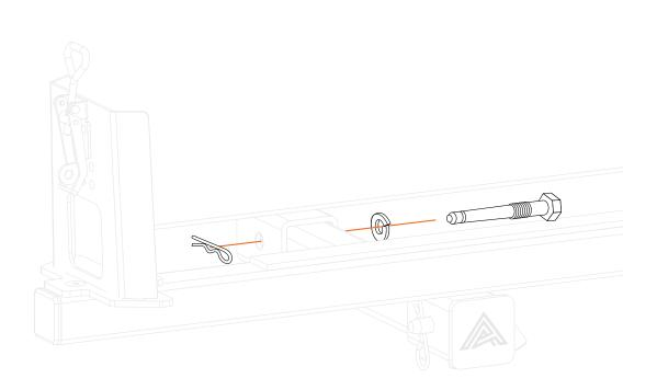
Insert the Silent Hitch Pin® into the receiver hitch and the Receiver Tube to reduce rattle.
