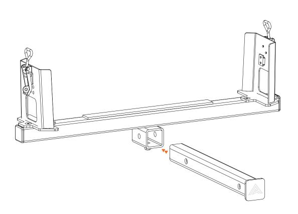
Slide the Receiver Tube through the collar of the Cross Tube.
