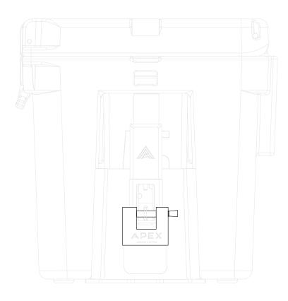
To fully secure your cooler into place, insert locks through each padlock hole near the lever. Note that the padlock holes can take up to a %" shackle diameter lock.
