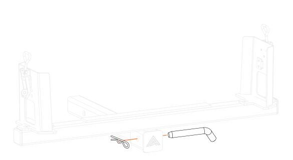
Slide the Assembly Hitch Pin into the round opening of the collar of the Cross Tube and the Receiver Tube.
