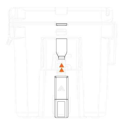
To further secure the cooler, place the Latch Cover over one of the latches. Insert the bottom of the Cooler Strap into the opening at the top of the Latch Cover.
