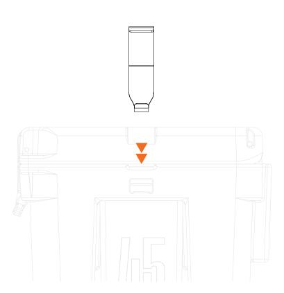
Slide the Cooler Straps through the slots on either side of the base of the cooler.
