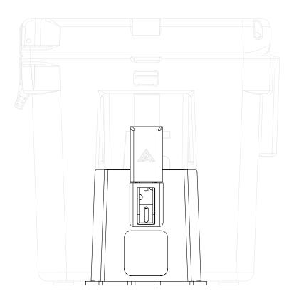
Pull the Latch up and hook it to the bottom of the Cooler Strap on either side of the cooler. Then, pull the Latch down on both sides of the cooler to secure the latches into place. The Latch Lever should rest on top of Latch Cover when snapped into place.
