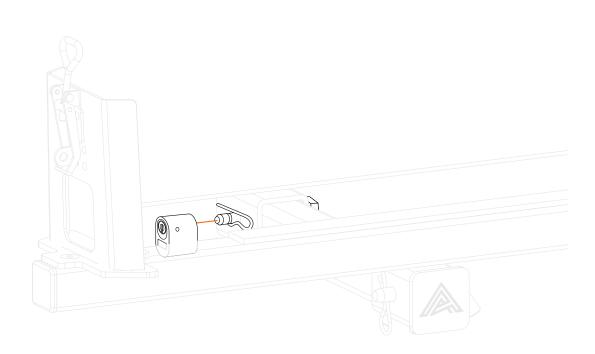
To further secure the Hitch Rack to the vehicle, install a lock on the Silent Hitch Pin.®
