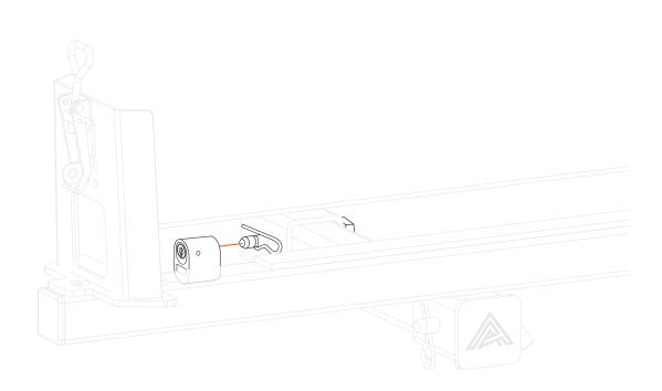
To further secure the Hitch Rack to the vehicle, install a lock on the Silent Hitch Pin.®
