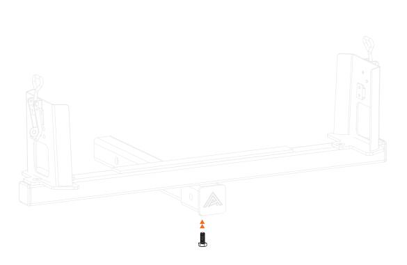
Tighten the Tension Screw and Lock Nut into the collar of both the Receiver Tube and the Cross Tube. This piece reduces movement between the Receiver Tube and the Cross Tube during cooler transport.
