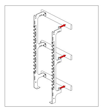
**STEP 4:** Recommended width between rack uprights is 41". (Optional widths: 41" - 47"). If you plan to use a bolton stall bar, 41" width is required.
