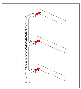
**STEP 2:** While person 2 holds one Off Grid Rack upright, vertically level, and flush against wood support boards/ ground, mark pilot holes on your wood support boards using a marker/pen/pencil.
