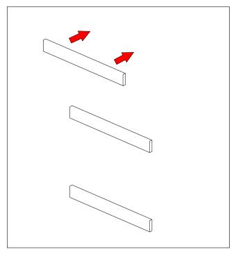
**STEP 1:** Install (3) 2x6" (or larger) wood support boards across your wall perpendicular to the ground using general wood screws at these specific heights:
