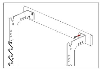
**STEP 5:** While person 2 holds the second Off Grid Rack upright, vertically level, flush against wood support boards/ground, mark pilot holes on your wood support boards using a marker/pen/pencil and secure 3/8" lag screws to to your support boards.
