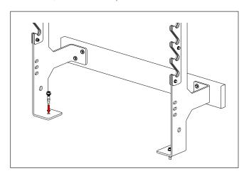
**STEP 6:** Secure your rack to the floor with (2) 1/2" concrete anchors.
