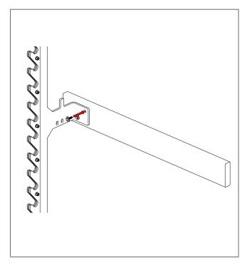
**STEP 3:** Install 3/8" lag screws to secure rack to wood support boards.
