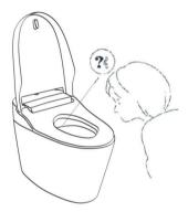
Please close the water valve and cut off the power and contact the seller when the water outflow.
