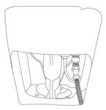
Confirm the inlet valve and reducing valve is open
