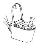
3.Dismantle the flange ring and gently press it against the water hole of the toilet bowl to make it stick. (Attached figure).
