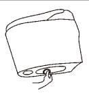
4.Lift the toilet bowl to make the flange ring center the water hole and place flat.(Attachhed figure).
