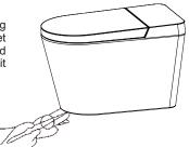
6.Install the water supply hose, and the hose must be tightly tightened with the angle valve. (Attached figure).
