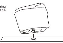
5.Apply waterproof glass glue, dealing evenly between the ground and the toilet bowl outline. It must be tightly sealed and cannot be used within 24 hours. It must wait until the glue completely cured.
