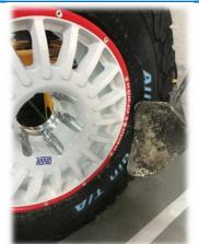
2. Before a new tyre mounting, the tightening area of the washers must be cleaned.
