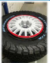
2. Then, the tyre can be mounted in its usual way. Once the tyre is inflated, with higher pressure than standard, we must tighten the tapered screws until they collide against the wheel. Only after all the screws are screwed in, we can proceed to restore the normal tyre pressure.
