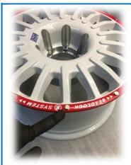
1. To mount the tyre all tapered 45 degrees screws must be previously removed.
