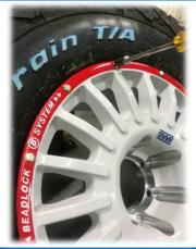
1. To dismount the tyre, first remove the screws from its lodge. Then dismount the tyre as usual.
