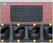
Optional: If preferred, fix a permanent 13-16mm irrigation system in place using the clips, according to manufacturers instructions. Use additional clips on spigots, if required.
