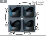
Seat each clip (may give loud 'snap' as seated). If a clip feels too stiff to push in, move on to the next one & continue to work ground the cell until all of the clips are secured.
