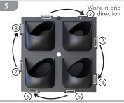
Seat each clip (may give loud 'snap' as seated). If a clip feels too stiff to push in, move on to the next one & continue to work around the cell until all of the clips are secured.
