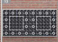
Install all of the remaining Fascias (steps 3-5) and spigots (steps 7-8) to complete the assembly of your G-WALL. Secure all remaining fixing spigots to the wall (step 11).
