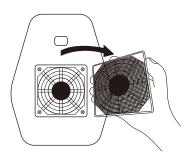
**3** Ensure the filter dry before installing
