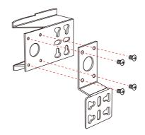
2. Attach the Motor Bracket Set on the outside of the grill's left side (or right, depending on the grill) with 1/4" Bolts & Nu t& Washers(L).
