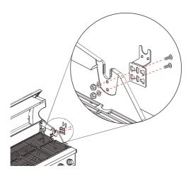
6. Mount the Motor (A) onto the Motor Mount (B).
