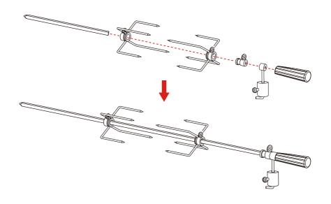
5. Attach the Rod Support Bracket(I) on the outside of the grill's right side with 1/4" Bolts & Nut & Washers (L).
