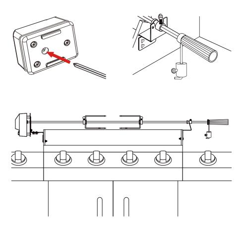
Using a combination of sections, securely assemble the spit rod to a length that will rest on both the Motor socket and the Rod Support Bracket.
