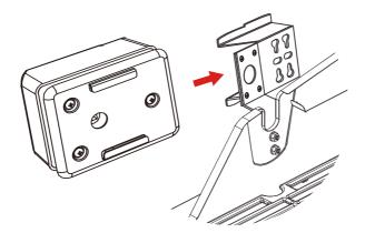
7. Slide Spit Rod into Motor socket, make sure the Rod Bushing(G) is resting on the Rod Support Bracket(I) and that Spit Rod is aligned properly with the rotisserie Motor(A).
