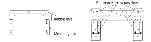
**NOTE:** Make sure the mounting plate is firm enough and flat against the wall after installation.
