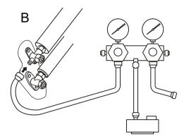
Connect the pressure hose to the service port and the manifold gauge to the vacuum pump.
