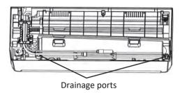
• Connect the drainage hose to the drainage port, and ensure the joint is firm and fully sealed. Wrap the joint firmly with insulation tape to avoid any leaks.
