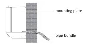
**NOTE:** The drain hose should slant downwards for drainage. Do not bent or twist.
