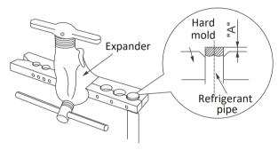
**NOTE:** The end of the pipe("A") must extend beyond the edge of the flare form in accordance with the dimensions shown in the table below.
