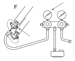
FIRST open the low-pressure valve for about 10 seconds and close. Quickly remove the pressure hose when the pressure indicates above 0.
