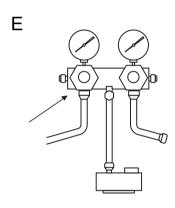
Close the low-pressure valve FIRST. Turn off the vacuum pump. Wait for 5 minutes, make sure the pressure change does not exceed 0.005 MPa.
