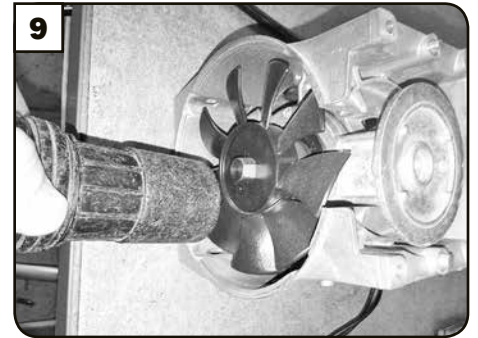
Gently pry off the fan guard. Blowout both open ends of compressor in a circular motion with shop vac or air nozzle.
