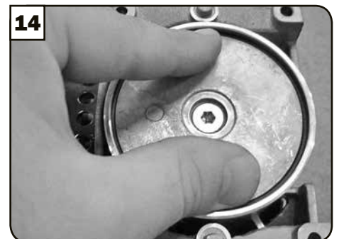
After tightening all the way down back screw off one turn and try rotating retainer by hand - it should have very minimal movement. Tighten back to torque spec.
