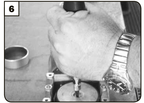
Remove retainer screw [C] using impact wrench with Philips Screw head or T-27 Torx star key. If it won't budge, heat screw center for 60 sec with torch.
