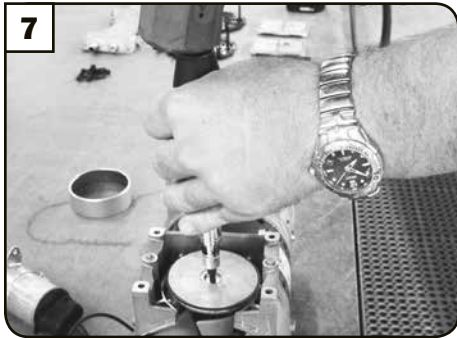
Immediately hit impact wrench with impact hammer until screw breaks loose. If it does not loosen, repeat heat, then hammer.
