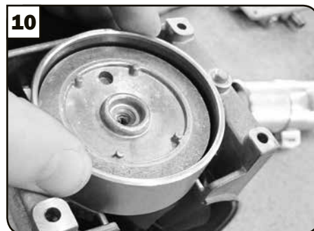
Raise piston rod to its highest point by rotating compressor fan on either side and now add new piston sleeve.
