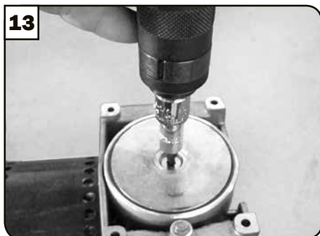
If using a torque wrench with Philips Screw head or T-27 Torx star key, use 100 inch-lbs. Be sure to align tab on the bottom of retainer with hole in rod
