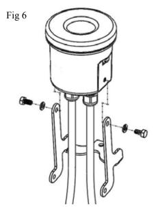
Important Note: Installation of the LED light fixtures on the above listed aerating fountain units with the mounting brackets oriented as shown will ensure proper submersion of the light fixtures. Each fixture must be partially submerged in order for lights to operate properly. Other applications for these fixtures must provide at least the same submersion to properly cool the fixture. Operating the fixtures out of water will damage the LED and void warranty.
