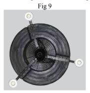
6. Using the cable ties, tie each fixture cord to bottom leg of mounting brackets using the holes provided. The will act as a strain relief and will keep the cord from being damaged by the fountain and balance the unit properly. Next, cable tie the main power cord to the float as shown in Fig. 10.
